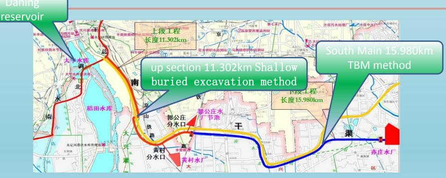
The length of Beijing south main canal is 27.3km, up section 11.02km designed in shallow buried excavation method, and down section 15.980km by TBM(tunnel boring machine)
